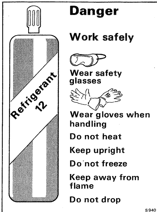
Fig. C3 Refrigerant handling - safety precautions
