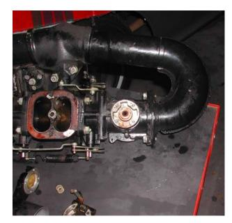
The last photo shows the float chamber removed and the diaphragm and jet removed.
