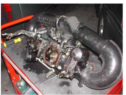
Replacement of the diaphragm on the larger engines is not major thanks to a simple fixing method of the induction system. The above picture is of a Cloud III which sprang a leak. Between the two carburetters there is a very long bolt that goes down into the engine. Having undone some pipes and the odd wire, this bolt can be removed and the entire induction system removed.
