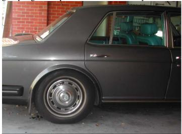
Sitting on its haunches having had its struts exhausted. Token springs that are holding this car up are there to avoid the Citroën malady of the car collapsing when the suspension fails.
