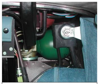
And here is what you will find having got the back of the boot uncovered. This is the right hand side showing the sphere and in front of it the battery switch which clearly needs to be moved to one side. The Factory recommends that the mounting block for the sphere (seen behind the coiled pipe) be removed to unscrew the sphere. This is unecessary as there is sufficient room to get the thing out without trauma. The left hand side is very accessable
