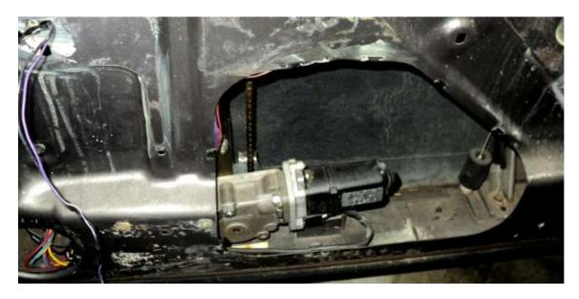
Well the door lining is off and there is the motor which is held onto the winding gearbox by just two studs and nuts. At lower left the broken coupler is emerging from the gearbox with the aid of your dentist's probe. Below that is a better view of the motor shaft adapter with a cross pin that engages the coupler and if you climb inside the door you can see a similar adapter on the input shaft of the gearbox.
