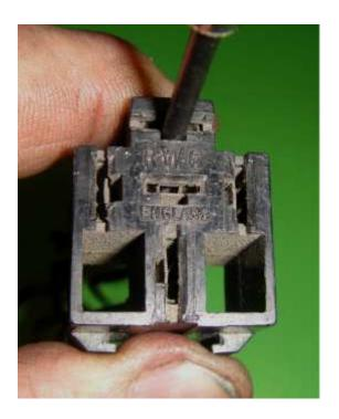
Removing the terminals and showing the tang that needs to be depressed before the terminal can be slid out of the block. The tool for depressing the prong I found most effective was a small electrical screwdriver. The right hand picture also shows the shoulders of the retaining groove that can be easily broken off by ham-fisted operators!
