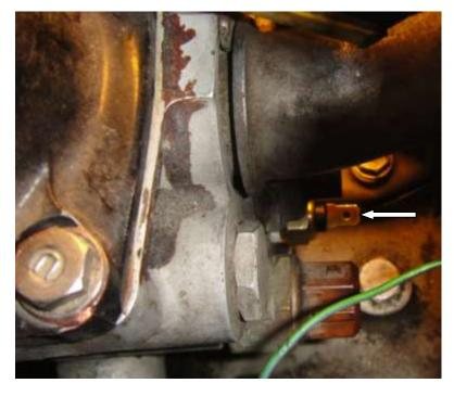
And here is the cause of low readings. The sender (arrowed) is simply a switch that varies in resistance indirectly as the temperature rises. Attached to it by a simple push-on connection is an active wire to the gauge. When the engine is very hot the resistance is low and power from this wire flows through the gauge and the switch to earth and the gauge reads high.
