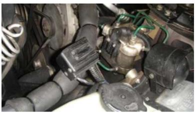
The above is the gubbins for the ABS system (antilock brake system). The small grooved box lying on the insulated air conditioning pipe should
