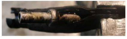
The restrictor being prised surgically out of the old bit of tubing.
