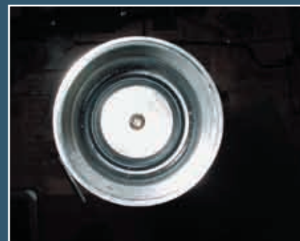
Below: End view of the main seal in-place.
