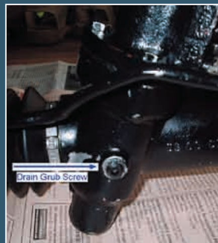
Above: The leaked fluid drain grub screw.
