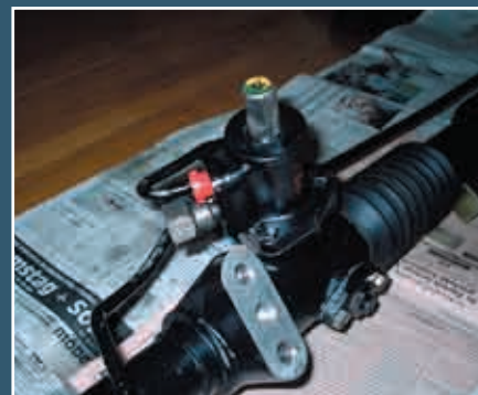
Above: The late-type rack, showing the cast mounts integral with the aluminium end housings and the external backlash adjuster. Early types have their mounts fabricated and welded to the end-housings.
