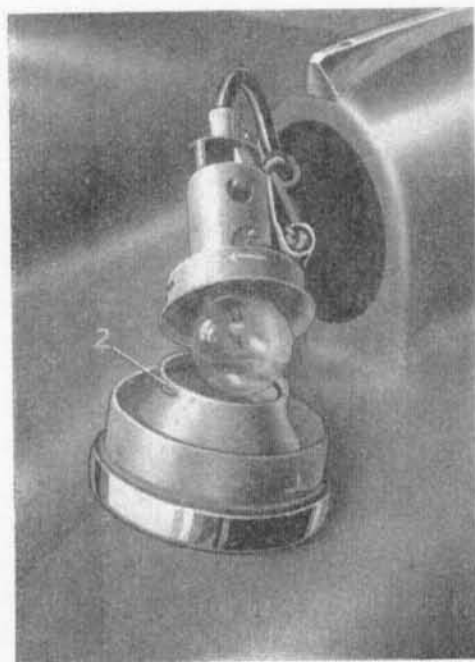
Fig. 49.—SIDE LAMP. 2. Spring catch.
