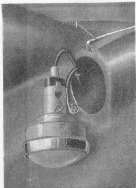
Fig. 48.—SIDE LAMP. 1. Locking screw.
