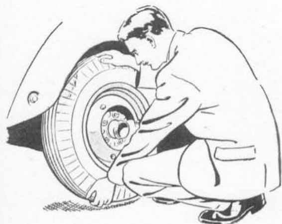
Fig. 31.—POSITIONING REAR WHEEL.
