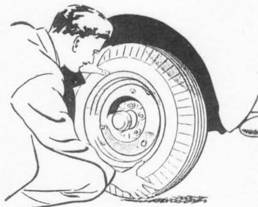
Fig. 33.—ENTERED STUD AT TOP.
