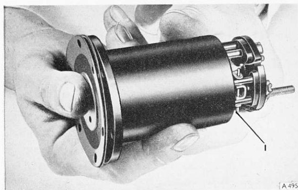
Fig. K6 Adjusting the diaphragm
