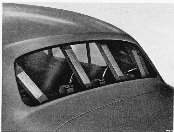
Fig. S49 Method of fitting clamps for pressing in the rear window glass
