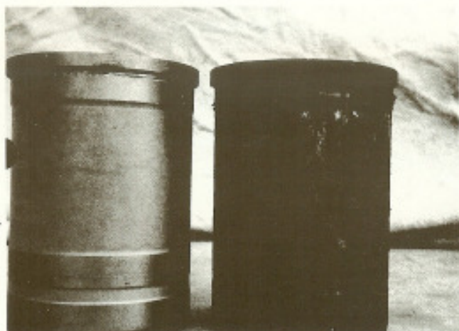
The old sleeve shows why the sleeves are often well-secured to the block. The build-up is basically aluminum corrosion.
