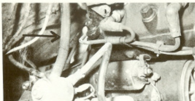
Be certain to remove the metal fuel line leading from the frame to engine (see arrow).
