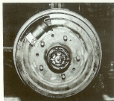
Figure 8: Front brake assembly after overhaul, but prior to refitting. Observe correct placement of bias springs—behind carrier plate. Figure 9: Brake shoes must be aligned square to the drum for maximum braking. Adjust the steady post: first screw it out part way, then adjust in with your square (made to size out of alloy) and a screwdriver. Figure 10: Brake drum with window cut out: this drum allows tightening of cylinder anchor bolts while brakes are on, thus centralized within drum. Handy here, it is a necessity for 4-shoe front brakes on Continentals. Be very careful when handling a brake drum. The cooling ribs are fragile and can be easily chipped—never hammer them.
