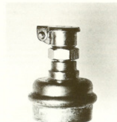
Figure 19: Rear brake equalizer and linkage. The pivot pin and bushes here were rusty, an indicator that the whole system, hydraulic and mechanical, requires attention. It is not enough to clean up this easily accessible unit and then stop. Figure 20: Author's modification: since there is no way to lubricate the pivot pin, I add an oil fitting to the cap over the pin. Then it's easy to put in a few drops of oil every time your car is serviced.
