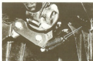
Mounting for u-joint holds driveshaft horizontal. Check for spring tension and rust. If the springs do not pull the shaft back, remove, clean, and refit, or replace springs as necessary.
