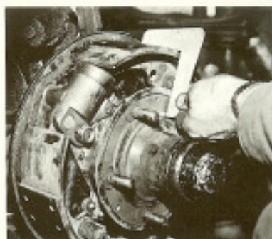
Figure 8: Front brake assembly after overhaul, but prior to refitting. Observe correct placement of bias springs—behind carrier plate. Figure 9: Brake shoes must be aligned square to the drum for maximum braking. Adjust the steady post: first screw it out part way, then adjust in with your square (made to size out of alloy) and a screwdriver. Figure 10: Brake drum with window cut out: this drum allows tightening of cylinder anchor bolts while brakes are on, thus centralized within drum. Handy here, it is a necessity for 4-shoe front brakes on Continentals. Be very careful when handling a brake drum. The cooling ribs are fragile and can be easily chipped—never hammer them.
