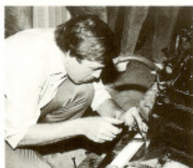
Left: Jim Shelly, NY, adjusts the exhaust valves on the RROC Foundation's R Type engine. Center: Even with the correct exhaust valve tool to keep the cam follower from turning as you adjust the valves (left, early post-war cars; right, R Type and Silver Cloud), access is extremely difficult when the engine is in the car. Right: Tool and wrenches in place for adjusting exhaust valves.
