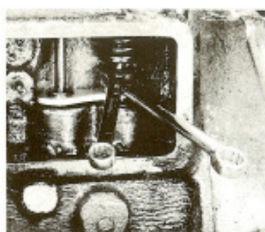
Left: Jim Shelly, NY, adjusts the exhaust valves on the RROC Foundation's R Type engine. Center: Even with the correct exhaust valve tool to keep the cam follower from turning as you adjust the valves (left, early post-war cars; right, R Type and Silver Cloud), access is extremely difficult when the engine is in the car. Right: Tool and wrenches in place for adjusting exhaust valves.
