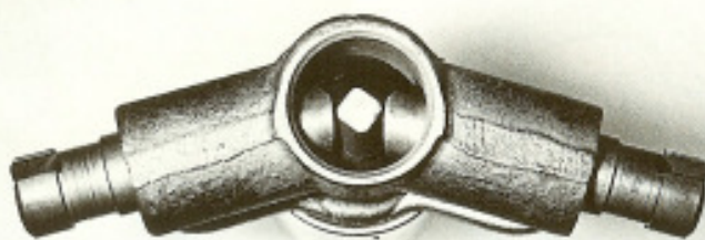
Figure 13: Rear brake adjuster unit plungers. They really are right and left handed. The notches fit locating pegs machined on the two bolts holding the adjuster to the backplate. Figure 14: Rear brake adjuster unit. If handed plungers are interchanged, the shoes will not contract enough to allow the drum to be refitted. When assembled correctly, turning the adjusting screw will produce an audible click.
