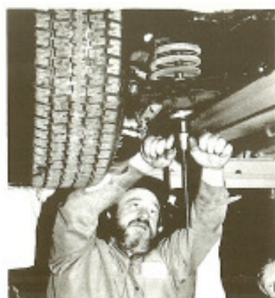
Doug Seibert, NY, compresses an SCI front spring to relieve pressure from the front suspension while he checks components for wear.
