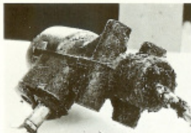
Figure 15: Master cylinder immediately on removal from car. Grit and muck indicate seepage and leakage—clearly time for overhaul. The muck is the result of a mixture of brake fluid and water attacking die-cast aluminum. Despite all the corrosion, these brakes worked, though they did not retract. You can inspect for corrosion without removal or disassembly: just look under the rubber covers. Figure 16: Master cylinder, exploded view. Notice corrosion on plunger at top right. Either fit replacement cylinders or bore and sleeve the old ones: cost considerations may dictate the method of repair.
