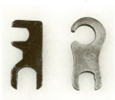
Left: Jim Shelly, NY, adjusts the exhaust valves on the RROC Foundation's R Type engine. Center: Even with the correct exhaust valve tool to keep the cam follower from turning as you adjust the valves (left, early post-war cars; right, R Type and Silver Cloud), access is extremely difficult when the engine is in the car. Right: Tool and wrenches in place for adjusting exhaust valves.
