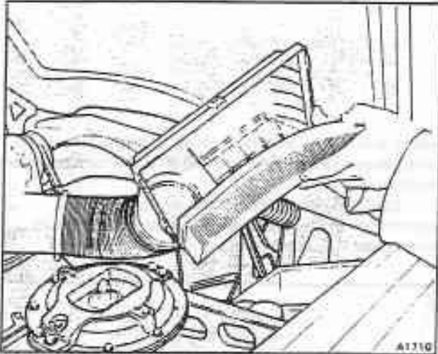
Fig.J3-2 Renewing the air filter element
