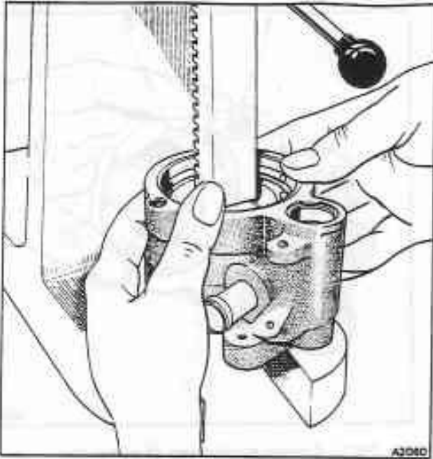
Fig. N3-9 Method of replacing end plate
