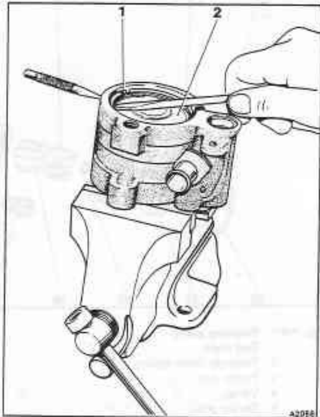
Fig. N3-4 End plate removal
