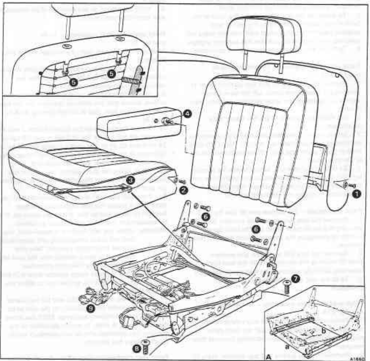
Fig. S13-1 Front seat trim and mounting arrangement
