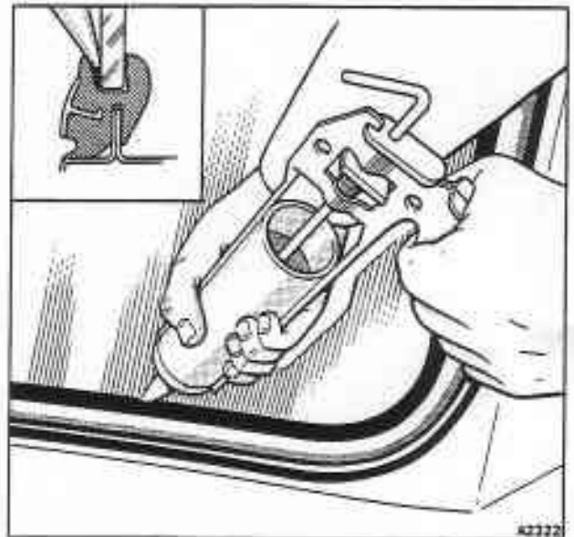
Fig. S24-4 Applying sealant between the seal and the glass
