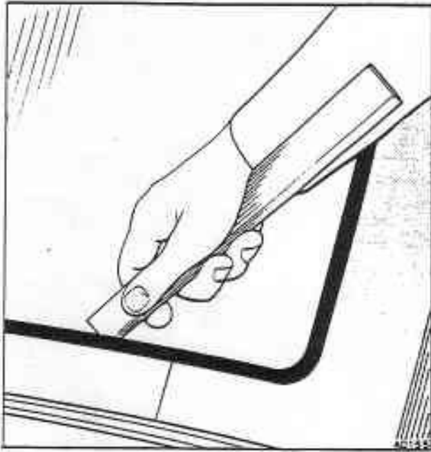
Fig. S11-10 Releasing the rear window from the seal
