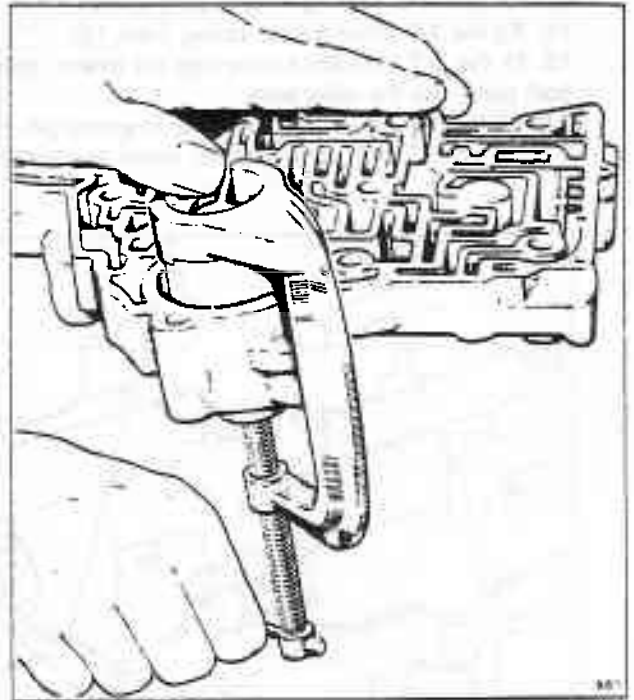
Fig. T12-14 Fitting the front accumulator piston and spring
